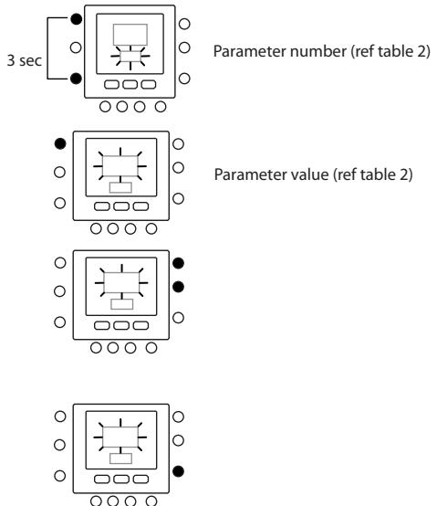
Press mode (M) button, the parameter value will be flashing in the temperature-zone of the display.
